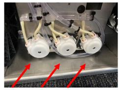
**2)** Depress the 2 finger tabs located on the side of the impellers. Gently pull the impeller off the spindle which extends into the impeller.
