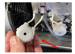
**3)** Using your thumb and forefinger, turn the spindle 20 turns to the left and 20 turns to the right. The impeller should turn freely. If significant resistance is present, note which pump is presenting the problem.
