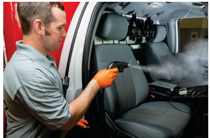
Disinfectant applied by APA hand sprayer from the AeroClave RDS 3110 to the cab and exterior of a rescue.
