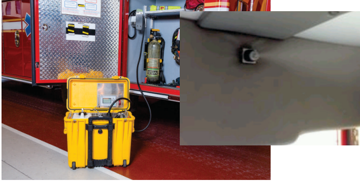
LEFT: The RDS 3110 unit connected to a rescue through the ADP-PT hands-free port. RIGHT: Nozzle inside patient compartment.
