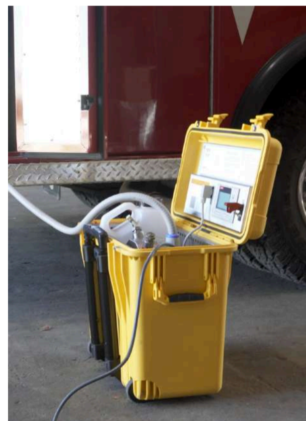
RDS 3110 connected to the ADP-PT hose assembly installed inside an exterior compartment.
